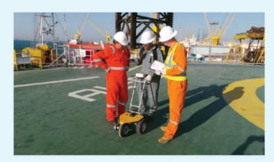
HFT is conducted using the latest friction measuring equipment micro Grip Tester (MGT). Our friction measuring devices and methodology meets all thestrict requirements under UK CAA, CAP 437 - Edition 8(December 2016). Those of us involved in the offshore industry know more than most about the importance of safe working and risk management. With this in mind, regular helideck friction testing gives offshore installation operators the assurance needed to remove helideck landing nets.
